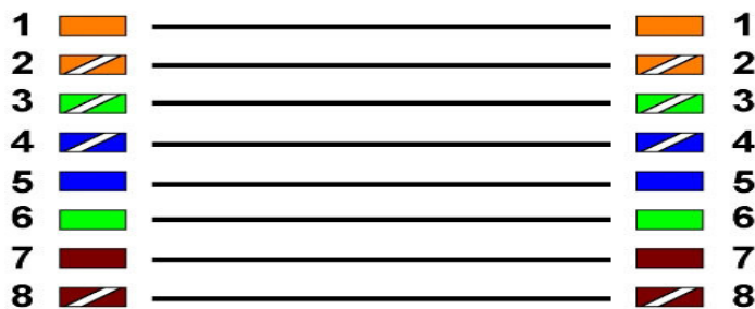
EIA/TIA T568B Straight Through Diagram
