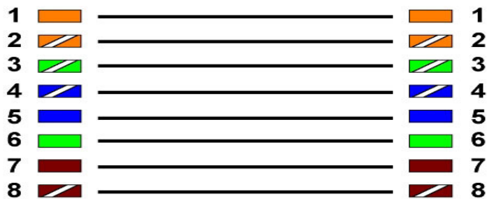
EIA/TIA T568B Straight Through Diagram
